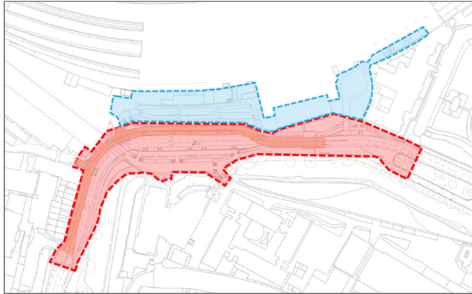
Figure 7.1: Diagram showing construction areas for Highway Works (red) & Station works (blue), indicating that both contracts could run concurrently. Note – temporary diversion road is within scope of Highway Works contract
